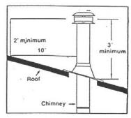
Chimneys shall extend at least three feet (3') above the highest point at which they pass through the roof, and at least two feet (2') above the highest roof structure or structure within ten feet (10') of the chimney.
