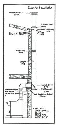
NOTE: In accessible areas, the exposed sections of the chimney must be closed off to avoid any contact or physical damage.
