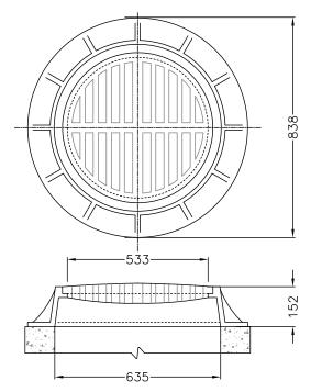
NO. 4 LANE PAVING CATCH BASIN MANHOLE FRAME & COVER
