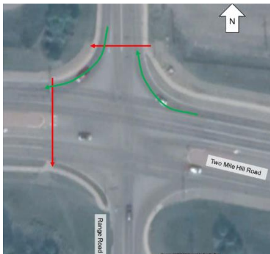
Figure 3-3 Conflicts due to Large Turning Radius and Visibility Obstruction
