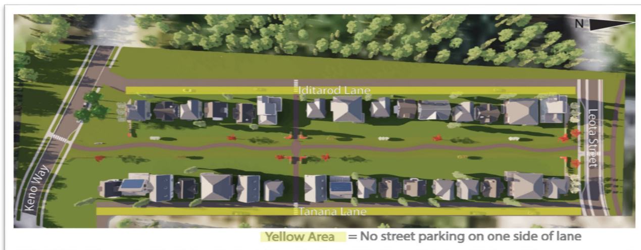
Figure 3 Design Option 2: Fire hydrants in lanes with a 3-metre paved Green Street
