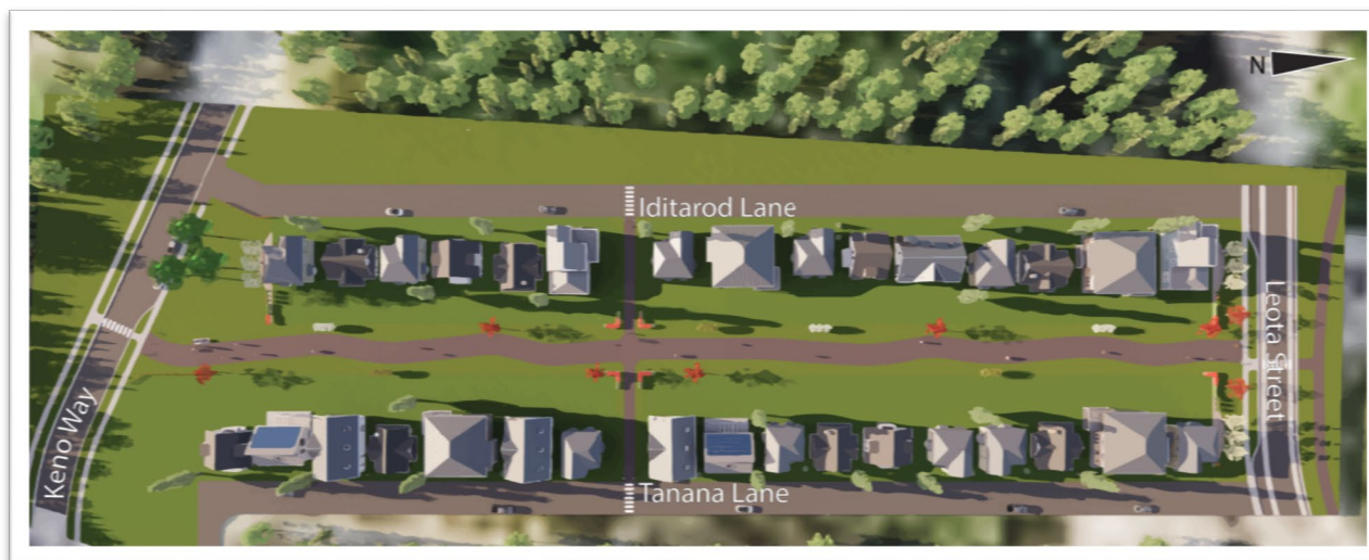
Figure 2 - Design Option 1: Fire hydrants remain with a 6-metre paved Green Street
